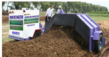
Tractor Mounted Rapid Compost Maker by Gurmail Singh Dhonsi, Sriganganagar, Rajasthan.
