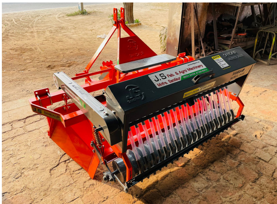
Tractor-operated multi-crop seed sowing machine developed for efficient and precise seed sowing for nursery raising.
