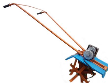
Battery operated weeder by Repalle Shanmukh Rao, Mahabubabad, Telangana.
