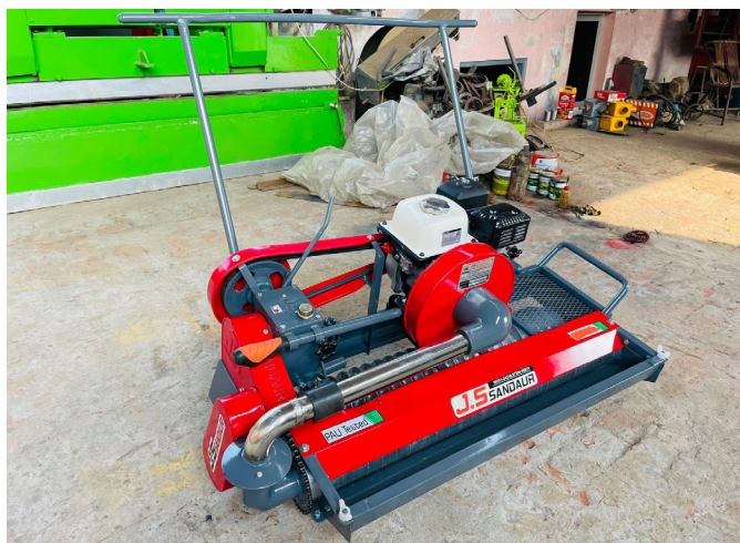
Pneumatic multi-crop seed sowing machine developed by Jaswinder Singh and field demonstrations conducted by the NIF team, for evaluating its precision and efficiency in nursery bed preparation and seed sowing.
