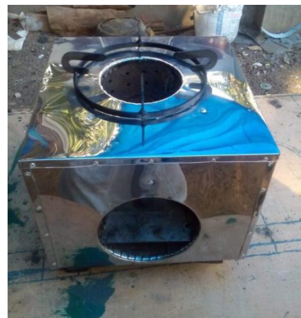
Improved wood stove with a secondary burning chamber by V. Jayaprakash, Calicut, Kerala.
