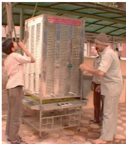
Solar-powered Natural Water Cooler by Arvindbhai Patel, Ahmedabad, Gujarat.
