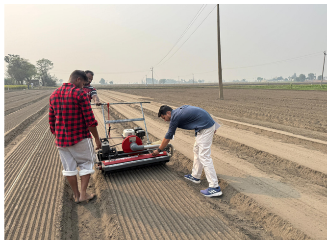
Pneumatic multi-crop seed sowing machine developed by Jaswinder Singh and field demonstrations conducted by the NIF team, for evaluating its precision and efficiency in nursery bed preparation and seed sowing.
