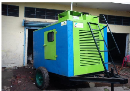
Trailer-mounted Biomass Gasification System by Rai Singh Dahiya, Jaipur, Rajasthan.
