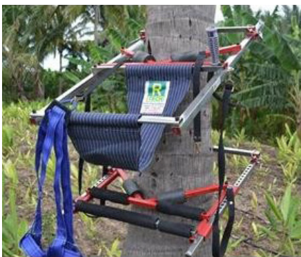
Multi Tree Climber by D. N. Venkat, Coimbatore, Tamil Nadu, in use on a coconut tree.
