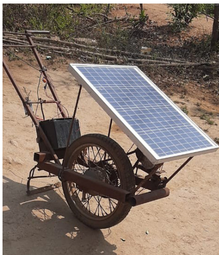
Single wheel solar powered weeder by Injapuri Anjaiah , Jagityal, Telangana
