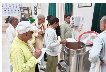
Participants observe an innovative vegetable-deseeding machine designed to efficiently extract seeds from surplus vegetables, creating an additional value stream for farmers.
