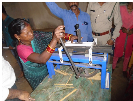
Dissemination of incense stick making machine at Dantewada
