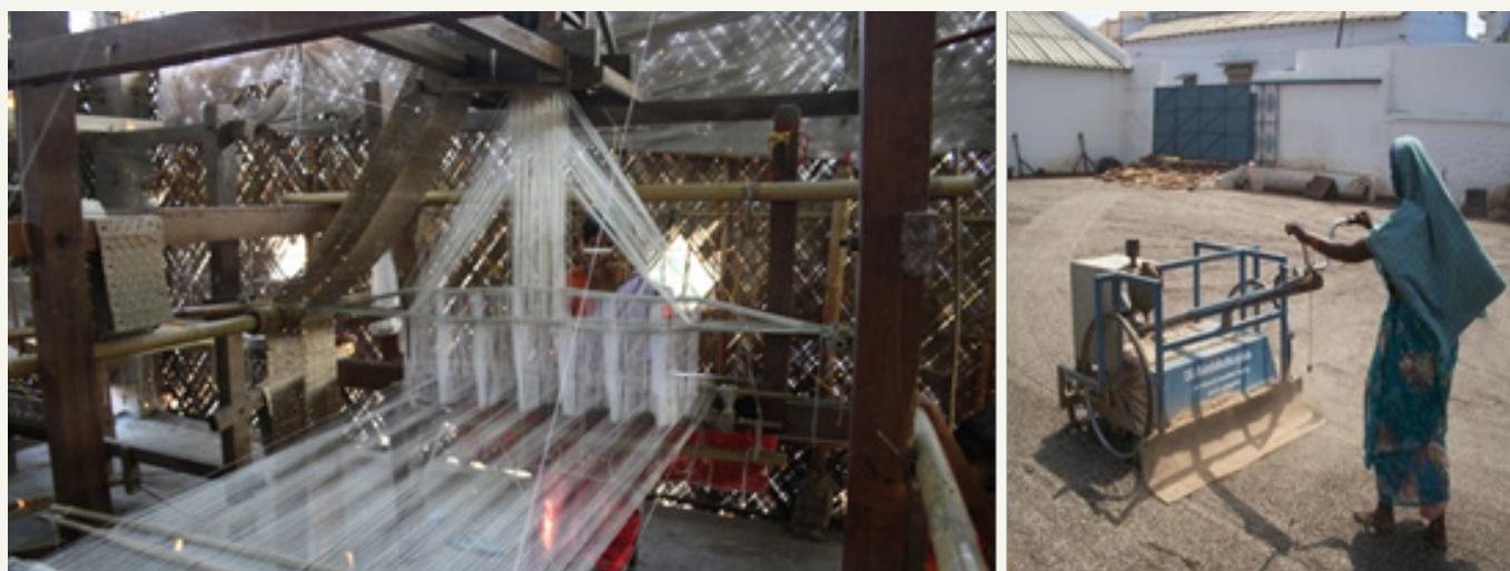
Fig 2. Reducing drudgery and enhancing efficiencies in rural micro industries (loom design making by weft insertion developed by Shri Dipak Bharali, Assam and parboiled paddy and oil seed turner developed by Shri R Ravi, Tamil Nadu)
