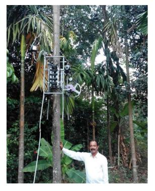
spraying attachment consists of pump and nozzle with pipe used to spray liquid pesticide on areca-nut tree. This device can be controlled through remote within a radius of 200m and needs two persons for installation.
