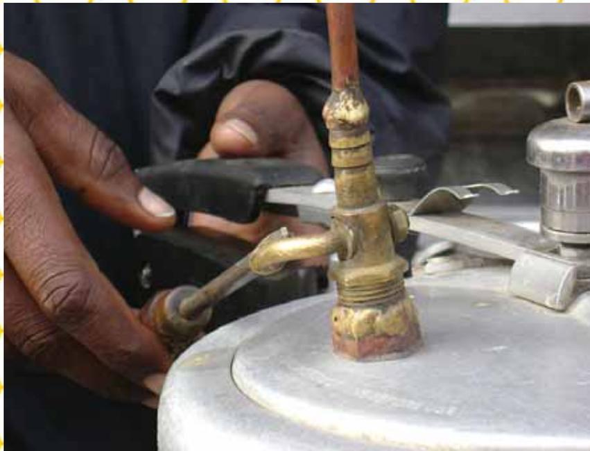
Conventionally, the pressure cookers have been used for making food only. However, Rozadeen (46) has modified the ordinary cooker to convert it into an espresso/cappuccino coffee making machine. The modified cooker is used to boil water and generate steam. Through a long delivery pipe having a regulator, high pressure steam is used to make frothy, tasty coffee.
