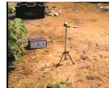
attachment for holding aerial fireworks (rockets) connected to the base and a hollow pipe for holding or guiding the fireworks.
