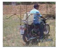
month long cotton-growing season and one acre of land (0.4 ha) requires roughly 300 litres of the mixture for spraying. This unit consumes three litres of diesel in three hours and can finish 1.5 acres at one go within an hour. The capacity of the tank is 70 litres.
