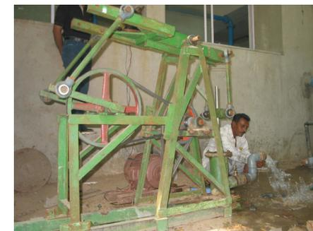
connecting rod. Prime mover (electric power or diesel engine), belt and pulley, revolute joints and bearings are also the accessories of the mechanism. The mechanism works on the principle of four-bar linkage mechanism having single degrees of freedom and there is a provision of balancing the load in the mechanism.
