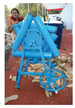
to the hulling operation. The frame is used to support the various components in the right position and all the rotational components are supported with the help of bearing blocks. The base of the frame is horizontally fixed to the floor by laying a machine foundation.
