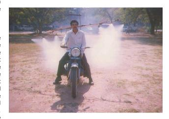
due to the inability to spray the fields quickly and effectively, the small farmers have their crops wiped out by pests. This motorcycle operated sprayer of Ganeshbhai's offers a solution to most of these problems.
