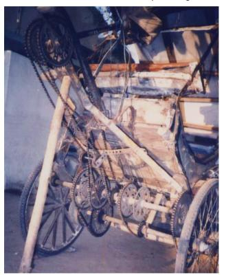
normal rickshaw where only one of the wheels is powered from the torque given by the puller. Whereas here by transferring it to both wheels, it became a "two-wheel" drive. The next stage in development was a four-gear rickshaw with differential mechanism and single axle in which the double-axle was removed and a single continuous axle was introduced. The power from the pedal was thus transferred to both the wheels, but in a much simpler fashion and it also reduced the add-on weight.
