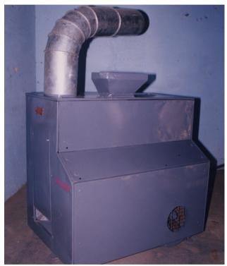
the peeling chamber are pushed by the pressurized air from the big blower to the rotating blade. The rotating blades hit the garlic cloves towards the serrated wall of the peeling chamber and there these get peeled. At the same time, the pressurized air from the big blower pushes out the dust and the skin of the garlic cloves through the exhaust pipe. The peeled garlic cloves from the peeling chamber are collected through the outlet
