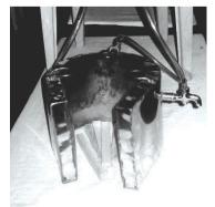
from the top into the tall drum placed on a stool behind the stove. In two hours up to 150 liters of hot water at 80 degree centigrade is made available in the drum. The entire unit is portable and can be set up anywhere. The cost is around Rs. 1000 because the water chamber of the stove is made of stainless steel to prevent rusting.
