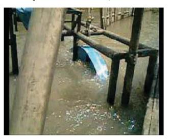
pump with guide blade is coupled in the turbine set for irrigation purposes. The driven gear with the help of a flat belt gives the required rotation of the pump for pumping water.
