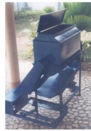
can thresh 600 kg of pepper per hour and a small model which has a capacity of 50 kg and can thresh 300 kg/hr. The average threshing efficiency observed is 90percent with only 2 to 3 percent damage.
