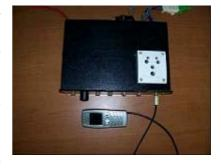
the device connected to it gets switched ON. It can be switched OFF by making another call from the same telephone. The calls made from un-identified telephones will not operate the switch.
