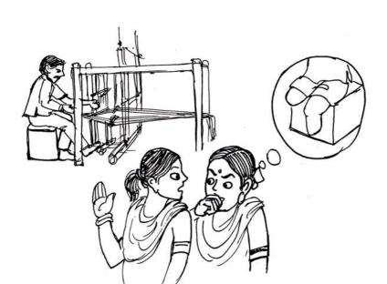
The two sisters have come up with a loom for lower limb physically challenged. In their loom, they have replaced the pedal operated system with a motor and a gearbox attached to a pulley mechanism.
