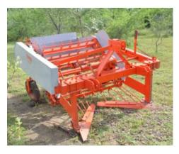
wheels have been provided at the rear to reduce the load on the tractor. Though the productivity of machine depends on the type of the soil, but on an average the machine can harvest about 3 to 4 Veegha (0.4 Acre) per hour.
