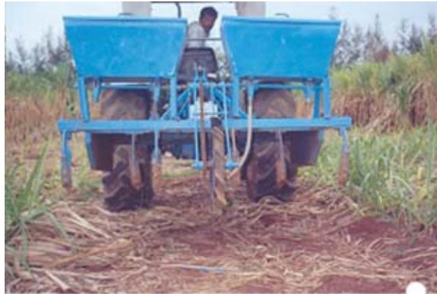
give the shaving effect on the sugarcane ratoon crop and manual cutting did not give uniform height. Ideally, farmers would like to have a machine that would do multiple operations such as stubble shaving, fertilizer drilling and earthing simultaneously. This would not only save time, cost and effort, by reducing number of
