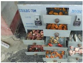
top, to dry various food items. The stove is a self-standing one, which also serves as doubling as a work place having a work platform at a height of 75 cm from ground and measures around 60 cm x 90 cm. Two cooking stoves have been provided at the top and a third one for drying purpose at the bottom in the centre.
