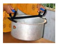
shafts are connected with semi-circular arc type plate and handle grip to hold edge of the utensil, which ensures safe lifting and usage. A set of two tongs can easily hold 10–15 kg weight.
