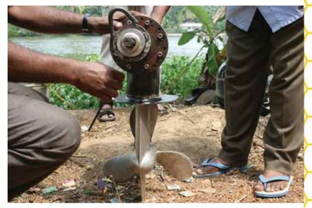
with inner spline cut with dual sided jaw and dog clutch. This provides smooth running and better power transmission for the marine diesel engines.
