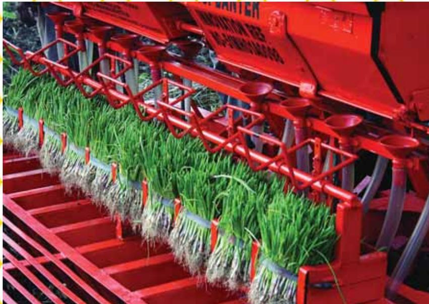
The task of transplanting onion seedlings manually is time consuming, labour intensive and toilsome process. PS More (66), a farmer and an innovator, has developed an affordable, semi-automatic transplanter for timely sowing of onion seedlings. He has also laid no restriction for anyone to copy and use his technology, and in fact wants the technology to diffuse widely for the betterment of the farmers.
