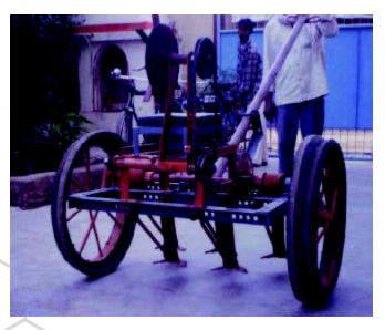
hand lever at the rear of this equipment. When the vehicle moves forward, it collects uprooted stalks, weeds and crop residue. When the lever is lifted, the collected material is dropped in to a heap to be carried away or burnt.
