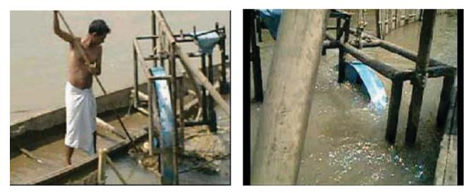
pump with guide blade is coupled in the turbine set for irrigation purposes. The driven gear with the help of a flat belt gives the required rotation of the pump for pumping water.
