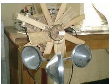
unique process basically improves the efficiency of the unit and sucks in and delivers more air. Due to the unusual arrangement of the two-layer blades, they develop vortex airflow, which results in higher amount of air/unit energy supplied as compared with single layer designs.
