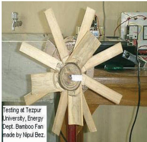
The significance of the innovation is in the arrangement of the blades and their placement, the angle of the blades with respect to the axis, the relative position of the smaller and bigger blades and the direction control of the fan for focusing and distribution of air. Each bamboo fan costs about Rs.100.
