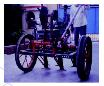
hand lever at the rear of this equipment. When the vehicle moves forward, it collects uprooted stalks, weeds and crop residue. When the lever is lifted, the collected material is dropped in to a heap to be carried away or burnt.
