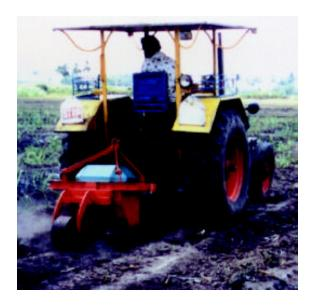
shrub-master (http://agricoop.nic.in), stubble shaver (http://agricoop.nic.in), etc. The shrub master, rotary mower and the stubble shavers has the swinging blades for cutting stubble/shrubs/grass. Weeding can also be practiced using these implements.
